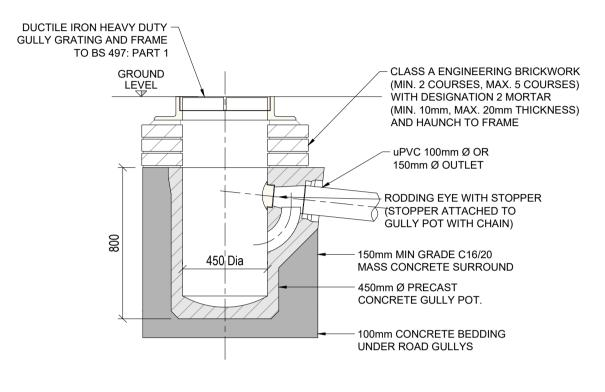
ROAD GULLY DETAIL SCALE: 1:20
